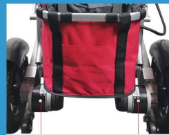
Motor 1 500W dual motor, DC motor /strong climbing ability
